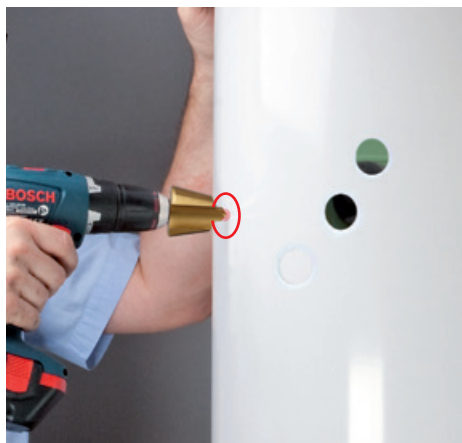
Drill the viewing ports with a sheet metal drill. The exact location of the viewing ports can be easily and precisely indicated using a visible EDM beam and can then be immediately drilled. The total station can remain in the housing for this.
