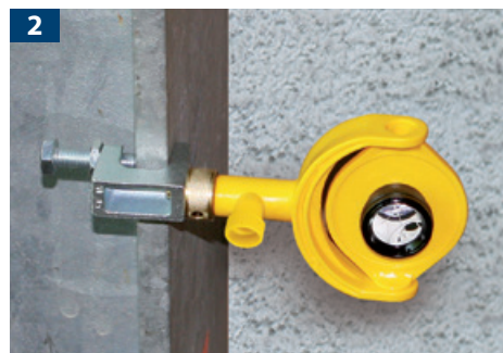
46-TK-M8 used here with the 11R5W adapter and 46-MP glass prism.
