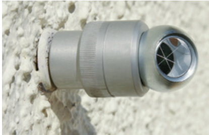
Ball prism monitoring system with M8 thread connection for mounting in a wall plug.
