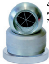
46-1463 with ball base 46-1460 and prism 46-1450
