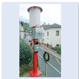
page 5 Measuring pillars for temporary monitoring campaigns and lockable lid
