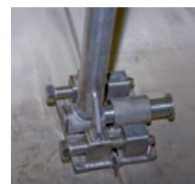
14-TK2 Detail clamping mechanism
