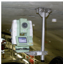
14-TK2: Overhead- mounting at the top of the tunnel
