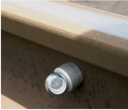
System of ball prisms consisting of a magnetic ball base and the ball prism as used in a track monitoring project.
