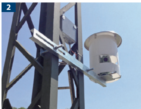
14-GMK Track measuring bracket for DB lattice masts
